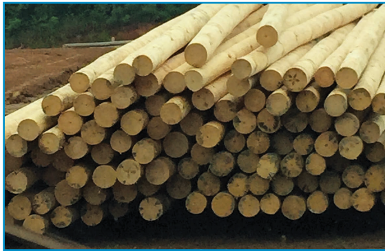
This operation not only peels poles for shipment as far away as Canada but also kiln dries poles to maintain quality of the shipped product as long as possible.
