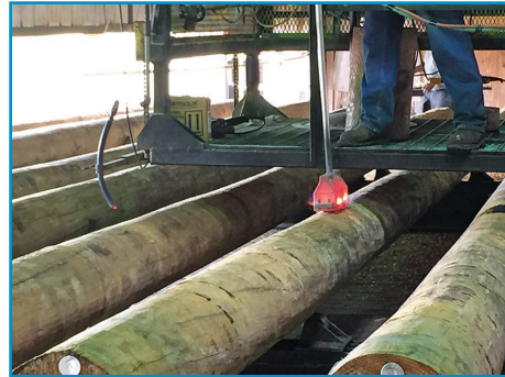
Cahaba is known as the largest single pole treating operation in the world. On the right is an example of pole branding.
